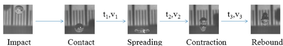
Figure 5. Schematic diagram of an impact cycle of an overcooled water droplet at different stages: impact, contact, spreading, contraction, and rebound.
